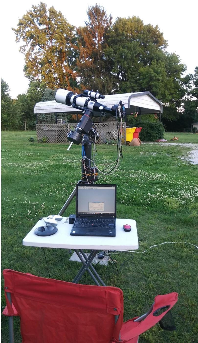
The St-8E, AR102 Telescope, T60 with docking station and Sirius Mount discussed later in the article. Note the cheap Xbox game controller to control the mount.
