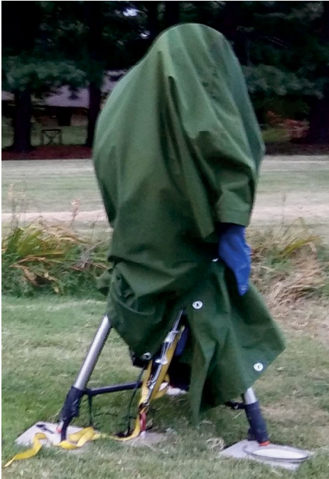
Image 2 - A large trailer hold-down screw and tie-downs secure the assembled CPC 1100 on paving stones, where a high-quality canvas protects it from the worst of the elements. Not the prettiest solution, but surprisingly functional.
