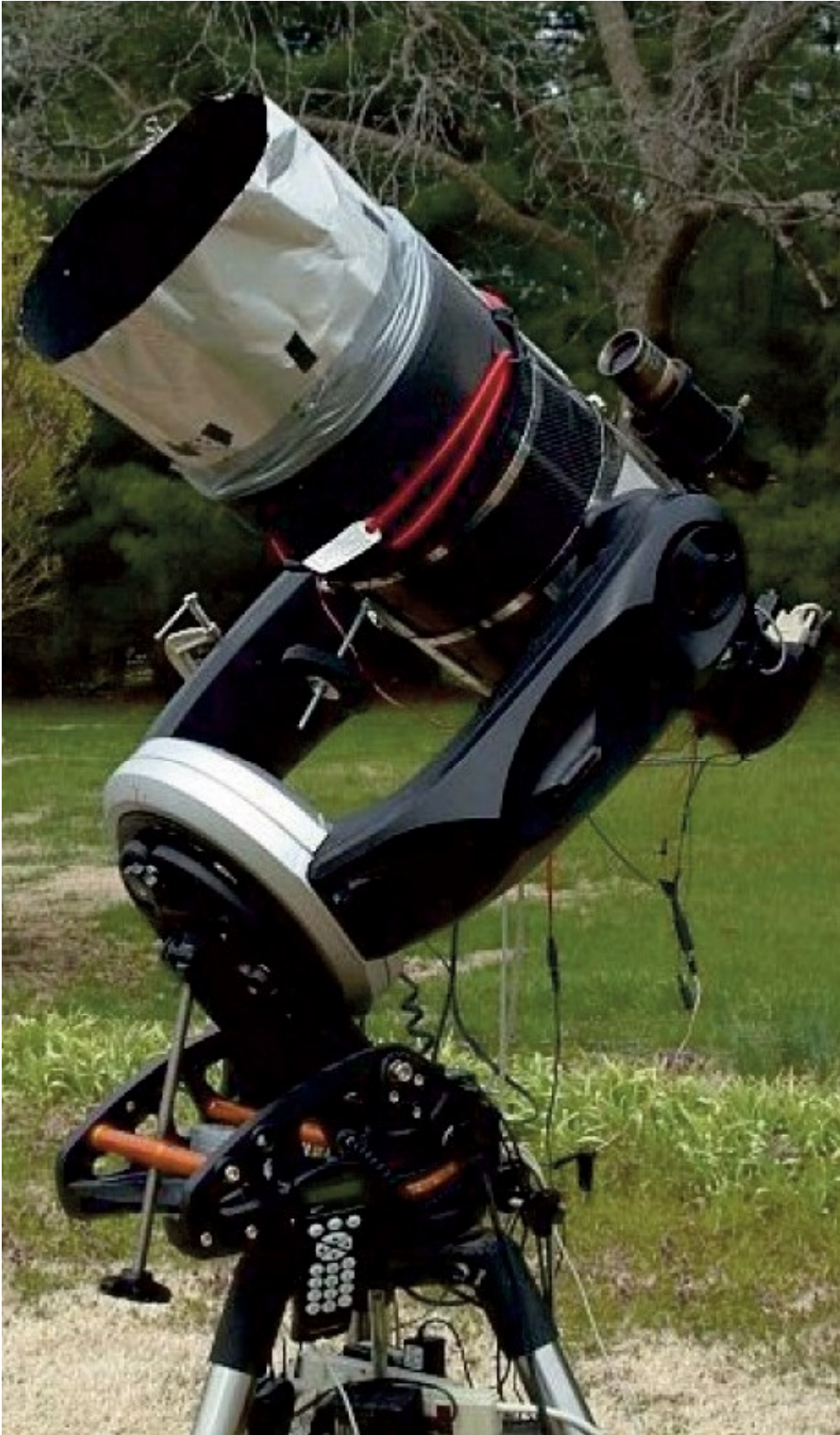
Image 4 - Celestron CPC 1100 (or Temple 28) with ST-8E camera, in all its duck-taped glory. The bungee cord and tape hold the filter material covering the vent holes. It looks messy but is now quite functional.
